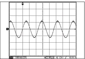
Figure 14: Input Terminal Ripple Current, i<sub>c</sub>, at full rated output current and nominal input voltage with 10µH source impedance and 47µF electrolytic capacitor (100 mA/div). See Figure 13.
