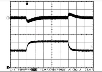
**Figure 11:** Output voltage response to step-change in load current (50%-75%-50% of Iout(max);  $dI/dt = 0.1A/\mu$ s). Load cap:  $10\mu$ F, 100 m $\Omega$  ESR tantalum capacitor and 1 $\mu$ F ceramic capacitor. Ch 1: Vout (100mV/div), Ch 2: Iout (10A/div).
