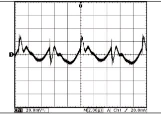
Figure 16: Output voltage ripple at nominal input voltage and rated load current (20 mV/div). Load capacitance: 1µF ceramic capacitor and 10µF tantalum capacitor. Bandwidth: 500 MHz. See Figure 13.
