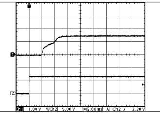
*Figure 10:* Turn-on transient at zero load current (2 ms/div). Ch 1: Vout (1V/div). Ch 2: ON/OFF input (5V/div).
