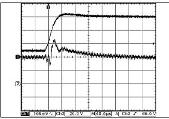
Figure 17: Output voltage response to step-change in input voltage (50V to 100V in 40µs). Load cap:  $10\mu$ F, 100 m $\Omega$  ESR tantalum capacitor and 1 F ceramic cap. Ch 1: Vout (100mV/div), Ch 2: Vin (20V/div).
