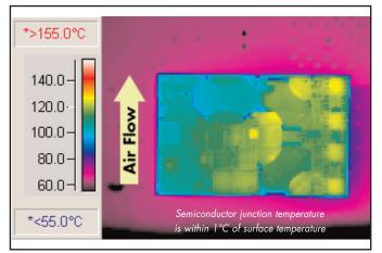
*Figure 6*: Thermal plot of converter at 40 amp load current with  $55^{\circ}$ C air flowing at the rate of 200 LFM. Air is flowing across the converter from pin 3 to pin 1 (nominal input voltage).
