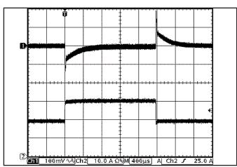
**Figure 12:** Output voltage response to step-change in load current (50%-75%-50% of Iout(max):  $dI/dt = 1A/\mu s$ ). Load cap:  $470\mu F$ ,  $30 \ m\Omega ESR$  tantalum capacitor and  $1\mu F$  ceramic cap. Ch 1: Vout (100mV/div), Ch 2: Iout (10A/div).
