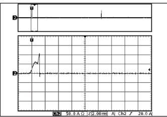
Figure 18: Load current (50A/div) as a function of time when the converter attempts to turn on into a  $1 m\Omega$  short circuit. Bottom trace (2ms/div) is an expansion of the on-time portion of the top trace.
