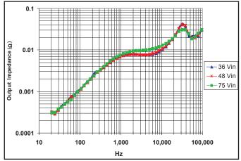
**Figure 19:** Magntiude of incremental output impedance  $(Z_{out} = v_{out}/i_{out})$  for minimum, nominal, and maximum input voltage at full rated power.
