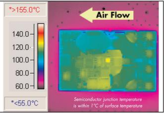
*Figure 8:* Thermal plot of converter at 40 amp load current with 55°C air flowing at the rate of 200 LFM. Air is flowing lengthwise from output to input (nominal input voltage).
