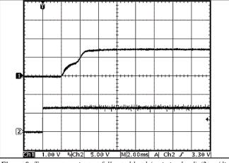
*Figure 9: Turn-on transient at full rated load (resistive load) (2 ms/div). Input voltage pre-applied. Ch 1: Vout (1V/div). Ch 2: ON/OFF input (5V/div)*
