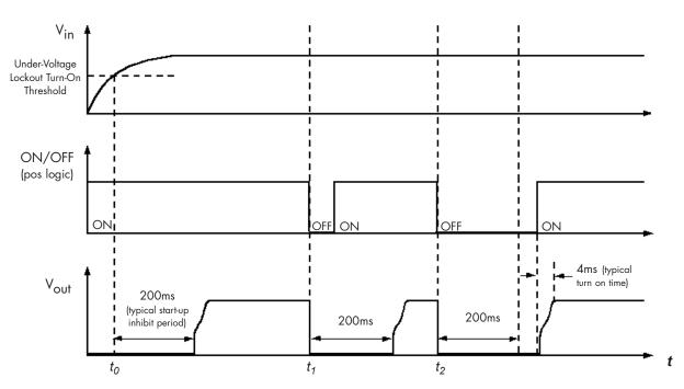
Figure F: Startup Inhibit Period (turn-on time not to scale)
