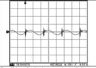
*Figure 15:* Input reflected ripple current, i<sub>s</sub>, through a 10 µH source inductor at nominal input voltage and rated load current (10 mA/div). See Figure 13.
